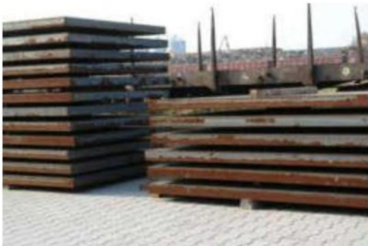
Steel plates shimmed with wooden bars
